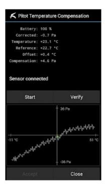
In case you have some doubt whether the drift compensation is good, you can use the **[Verify]** button. Just start and observe the graph while the temperature changes. Again, a curve for the residual drift will be drawn, but it should be very small, similar as my result:
