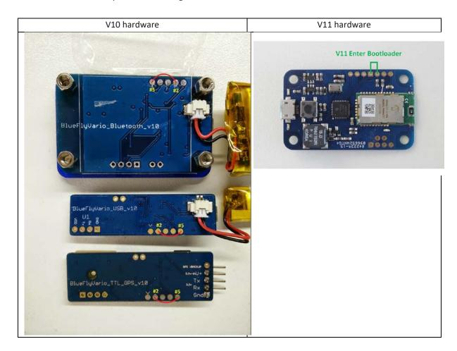
You will also need to establish a serial connection. You can test your serial connection using the BFV Desktop application or a terminal emulator like Realterm:
