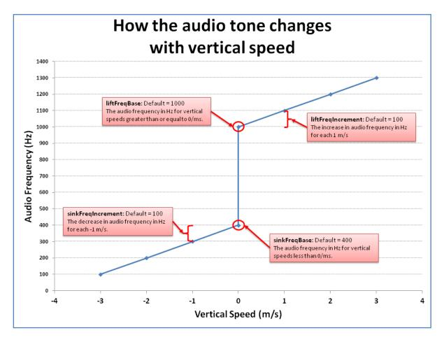
Note that in the most recent versions of the BlueFlyVario (from v7 onwards), the Audio Frequency cannot be played below 125Hz. If the combination of the settings and the measured vertical speed results in a calculated audio frequency below 125Hz the resulting sound will be clamped to 125Hz.
